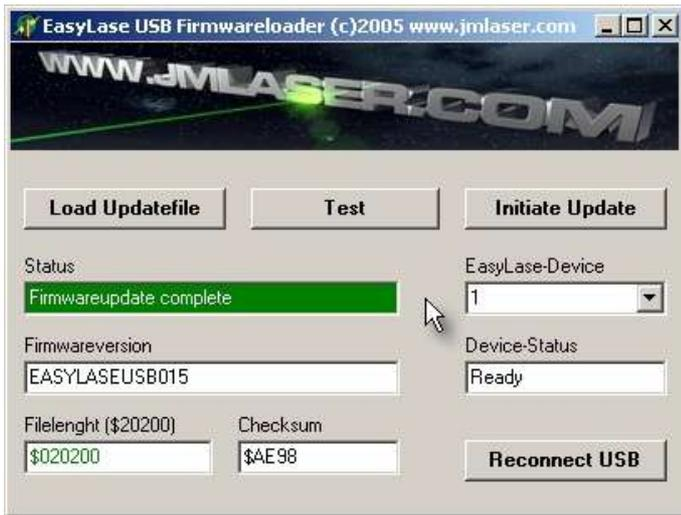
Now, another device can be selected using the selection-box and the update can be processed without any need to load the firmwarefile again.
