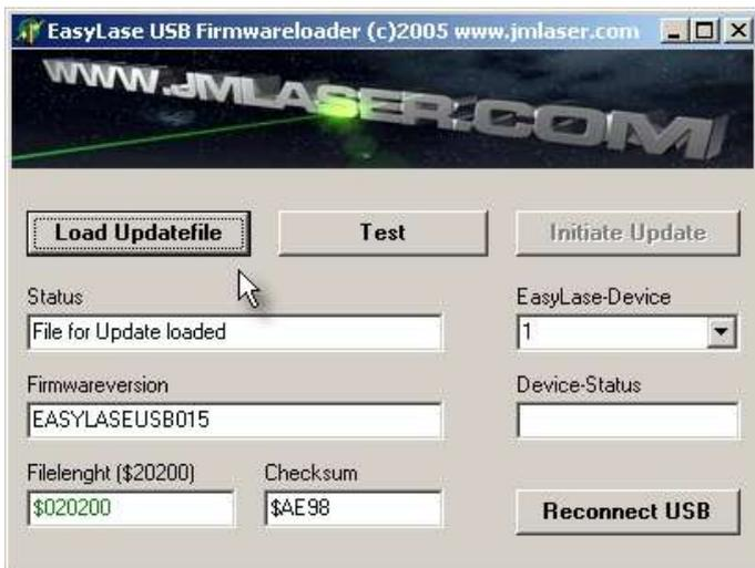
When a valid firmwarefile is loaded, the name and release of the file is displayed and the button to test the data communication is enabled.
